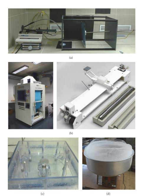
FIGURE 1: Spinning devices: (a) needle electrospinning with metal needle connected to the dosing equipment and high voltage source and grounded metal plat collector; (b) Nanospider™ for needleless electrospinning technology and string spinning electrode (arrowed); (c) centrifugal spinning laboratory device with rotating disk and eight collecting cylinders arranged in a circle; (d) machine for cotton candy production The Breeze® 3030EX used for melt centrifugal spinning.
