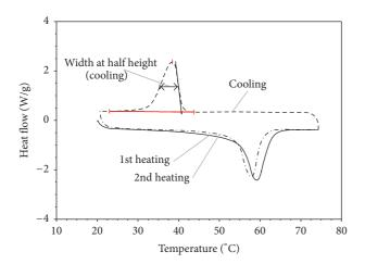
FIGURE 4: An example of DSC scan for one sample E (solution 24 wt% PCL45 needle electrospun from ethyl acetate/DMSO (8:2)) showing parts of the curve representing 1st heating, cooling, 2nd heating, and width at half height at cooling part of curve.
